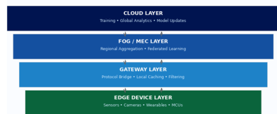
Fig. 1. Edge AI Hierarchical Architecture — data flows upward; model updates flow downward.
