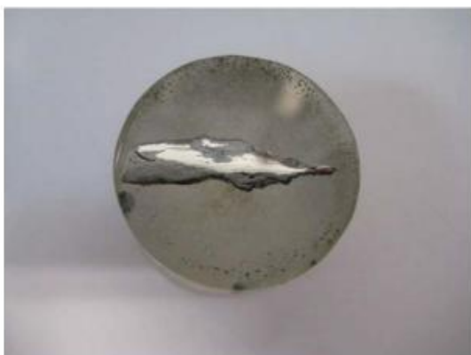
Figure 3: It was found that a steel nail had metalcore pieces inside it. Scanning Electron Microscopy (SEM) was used for the metallographic study.
